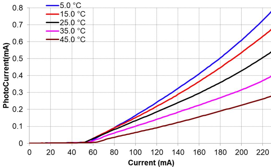
Figure 6: Monitor Photodiode Current versus Bias Current
