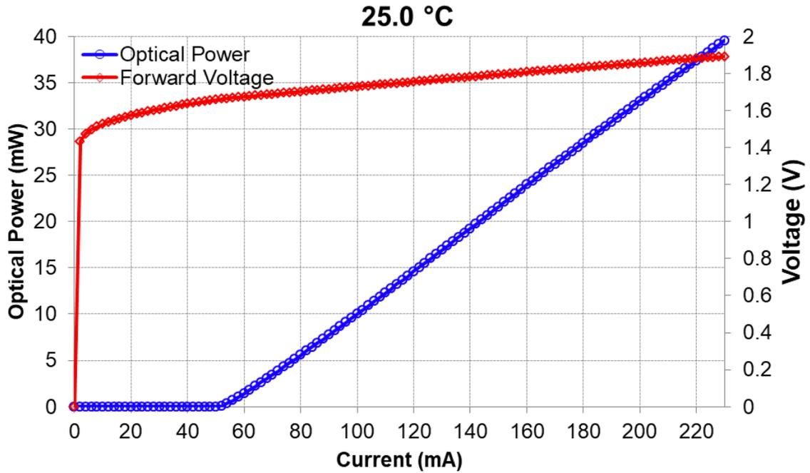
**Figure 1: Output Power and Operating Voltage versus Bias Current**
