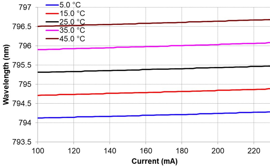
**Figure 3: Wavelength versus Bias Current**
