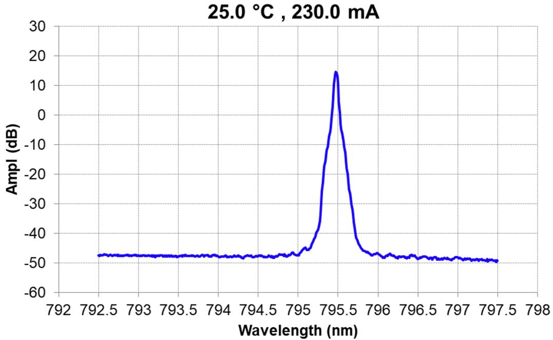
Figure 5: Optical Spectrum (RBW=0.02nm)
