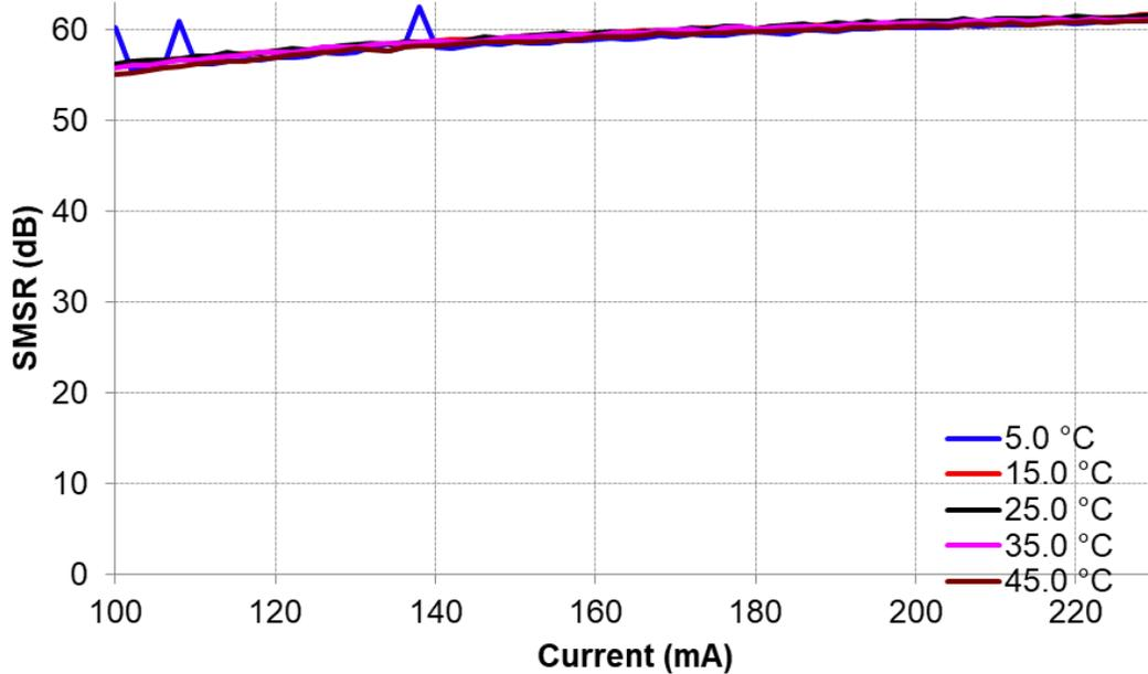
**Figure 4: Side Mode Suppression Ratio (SMSR) versus Bias Current**
